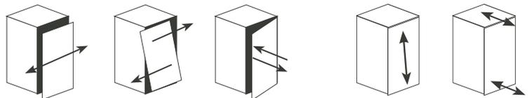
Horizontale, vertikale und axiale Justierung der Front. *The door position has three-way adjustment.*
